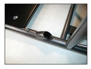
The driver side bottom rail has a cable openings at the front of the foot box and at the 4-link upright for master disconnect switch cables and the coil wire as standard equipment.
