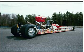
The XL Series body is a modular design with the main section (from the front spindle mounts to the driver area) being one piece, the rear panels and the removable nose are separate pieces. Constructed of fiberglass the body only weighs 38 lbs. and is virtually industructable. A fiberglass body is as light as an aluminum one, is stronger, doesn't dent and it is very easy to repair if you do damage it. The body can be completely removed or "flipped up" to work on the chassis.
