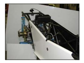
The rear body panels extend to the edge of the chassis 4-link mounting plates. We all know that decals are what pay when we win, this design gives you a much larger area for them. Notice also the rear panels roll around the top rail for added strength and to be "Quay" different.
