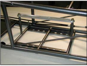
Dual battery mounts are standard. They are designed for dry cell altima batteries. Why dry cell? Have you ever had to clean up the mess a wet cell makes or had one quit because the plates hit one another... Enough said!!!
