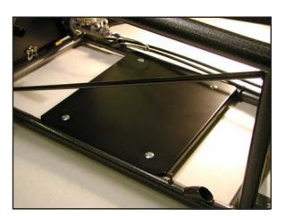
The electrical component tray is an aluminum dzus buttoned in plate forward of the foot box. Quick disconnect fittings would allow easy removal in case of ignition failure.
