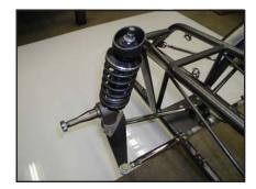
New for 2001 is a mini strut front suspension. This strut is manufactured by Strange Engineering to duplicate their "Pro Stock" strut only its lighter, shorter and has less travel. In our first tests the car ran mid 7.70's @ 174 mph, and the drivers quote was that "it was the smoothest car I've ever driven."
