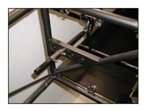
The throttle pedal stop is the strongest of any manufacturer. If adjusted correctly it stops cable breaking and erratic performance caused by pedal flex.
