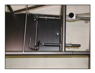
5" fully adjustable throttle and brake pedals are a XL series standard as well as a Tilton master cylinder mount.
