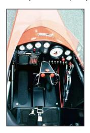
The dash area is larger and allows a much greater latitude in gauge and delay box placement. The electrical switches are in the dash as is the on/off cable ball for the master disconnect switch. The steering wheel is adjustable both in/out and up/down. Adjustable pedals are standard.
