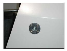
The body mounting buttons are a non captured button with reinforcing plates both inside and outside of the fiberglass. This doubling of the reinforcing plates gives a much stronger mounting area.
